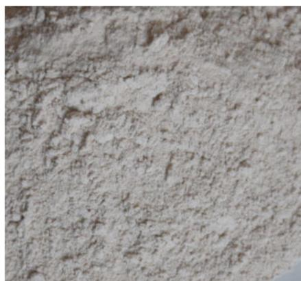
Magnesiumchloride flakes (MgCl<sub>2</sub>) are dissolved in water before mixing with CCM to create MOC.
